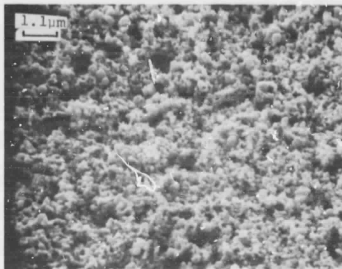
Figure 2. SEM micrograph at 1800x of F7 copper fluorocarbon paste fired at 600°C by the two step process.
